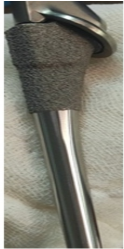
Figure 1: An example of a typical implant design of a reverse shoulder prosthesis featuring a proximal metaphyseal coating with a distal polished component.
